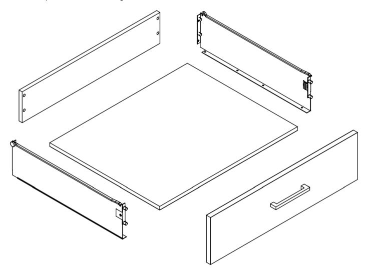
Note that the laminated bottom panel is supported by the steel flange on each of the steel drawer side panels and is screwed in place.
